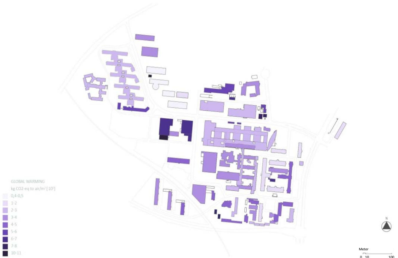
FIGURE 25 – MAPPING OF THE GLOBAL WARMING POTENTIAL PER SQUARE METER, IN CO 2 -EQUIVALENTS TO AIR, OF ALL BUILDINGS AT OUH
