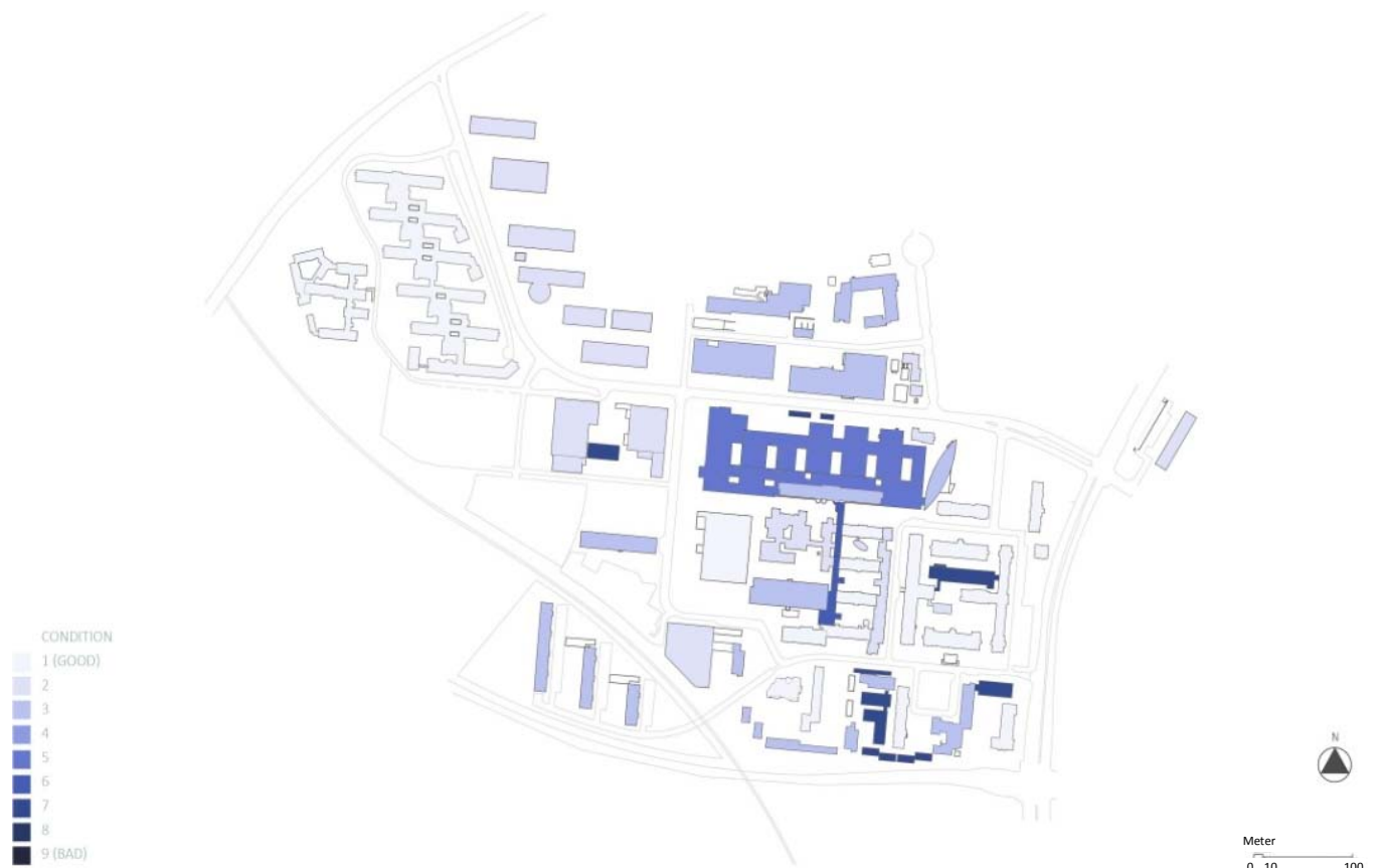
FIGURE 12 – MAPPING OF THE CONDITION OF THE BUILDINGS AT OUH ACCORDING TO THE SAVE-METHOD
