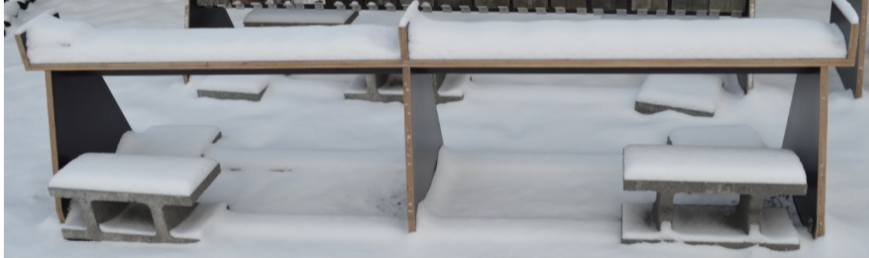
Figure 4.20: Picture of the specimens, horizontally oriented, without shelter, covered by snow
